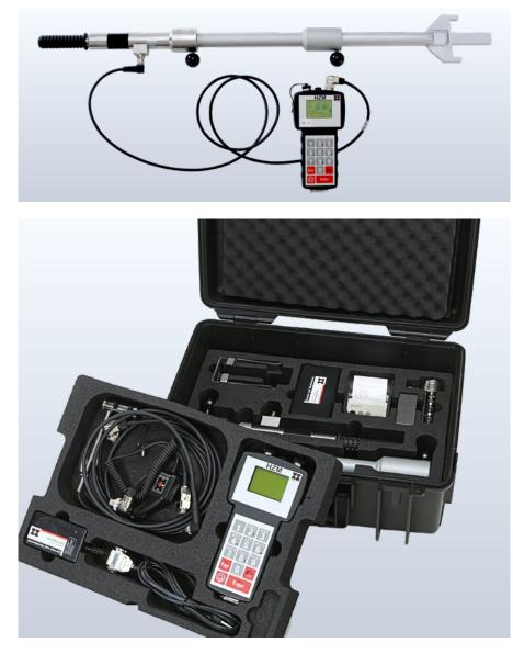
Manual setting forces on all HAN-NING & KAHL point machines can be measured using the HZM measuringsetting lever and the HZM force-measuring device.
